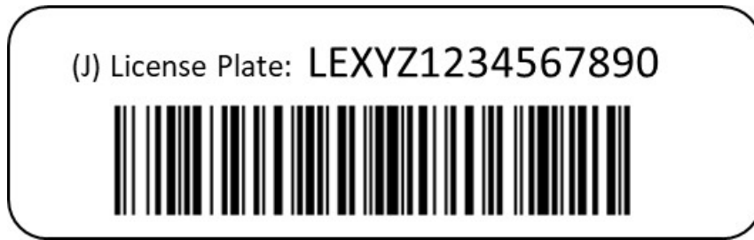
Figure 2 - License Plate Number encoded in a Code 128 symbol
