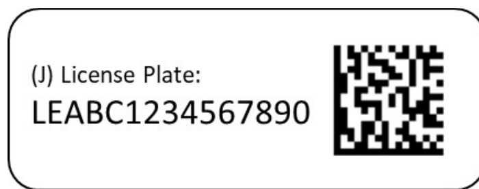
Figure 3 - License Plate Number encoded in a Data Matrix symbol
