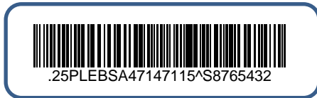
Figure 7 - Example Code 128 with two ASC DI headed data elements concatenated by separator “^”
